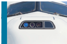
Camera equipped with multi-spectral sensors on aircraft nose
