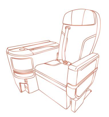
Individual seat with side console and built-in stowage
